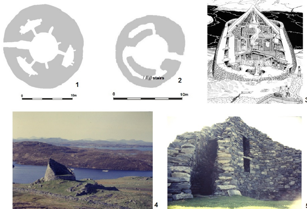
1: - Ground Plan of the Broch of Mousa, Shetland. 2: - Ground plan of Dun Bharabhat, Lewis 3: - Reconstruction drawing of Dun Carloway. Courtesy & copyright Alan Braby. 4: - View of Dun Carloway, Lweis Courtesy & copyright Alex Gibson. 5: - Detail of the cavity wall at Dun Carloway. Courtesy & copyright Alex Gibson.
